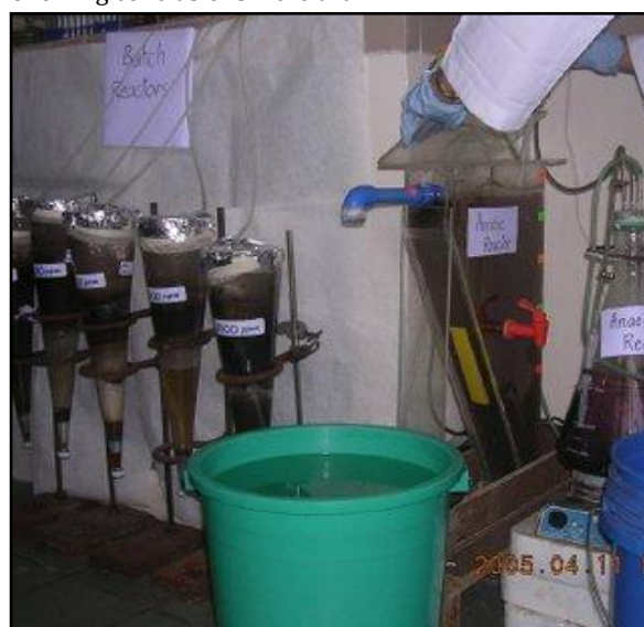
Fig 06: Aerobic and anaerobic reactors
