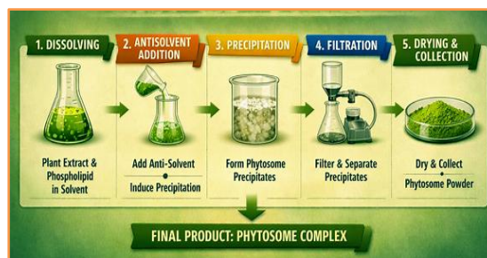
Figure 02: Flow chart of anti-solvent precipitation method
