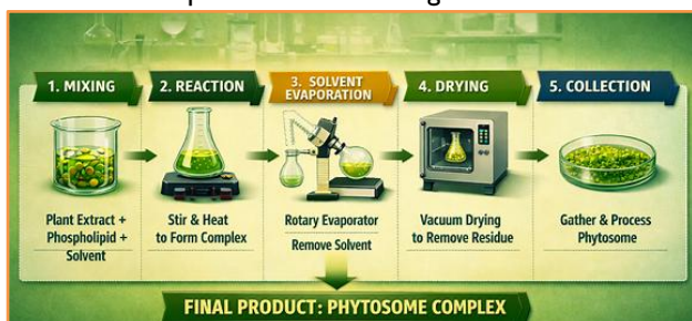
Figure 01: Flow chart of solvent evaporation method
